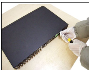
①disassemble the screw
