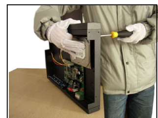
③fix the screw of hard disk
