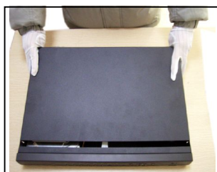
②disassemble the cover
