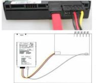
Your HDD should be installed inside the DVR. Please connect the HDD in the standard way, screwing the HDD into the HDD brackets or DVR base. All necessary cables are delivered with the DVR. Use instructions that came together with the hard drive for exact wiring and installation. Please connect the power cable to the appropriate socket, and the data cables to their corresponding connectors.
