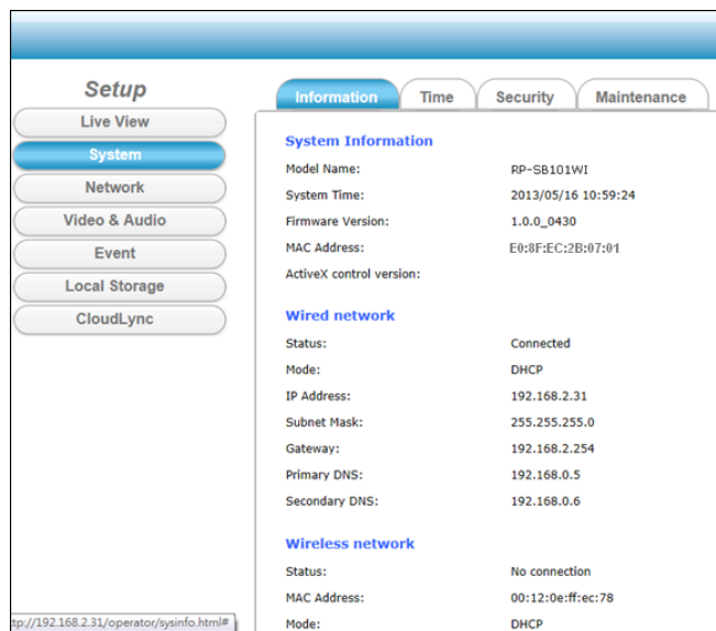
Figure 2-2 “System Setup” Tabbed Panes
