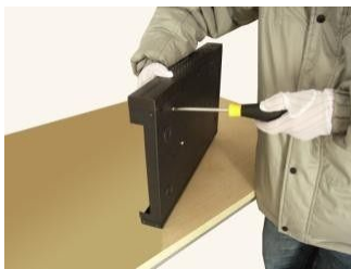
④fix the screw of hard disk
