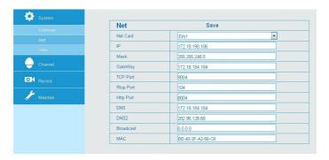
In this interface we can set the internet attribute of device, IP address, subnet mask, gateway and preferred domain server included. Make the internet configuration according to the actual situation.
